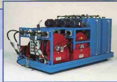
This lube pallet contains a 4-product lubrication system, electric pumps, and retractable hose reels with totalizing metered dispensing handles for use on any motorized vehicle.
