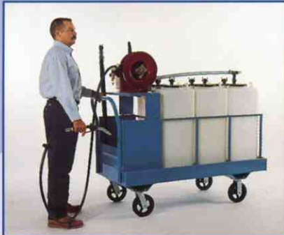
This 3060 lubrication cart holds 6 products (each in 15-gallon container) and features an air-operated diaphragm pump with a retractable hose reel with dispensing handle.
